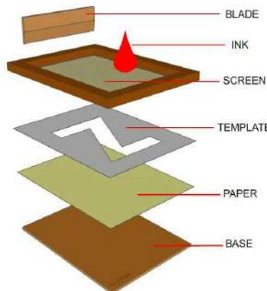
1. The paper to be printed on is placed on top of the base.
