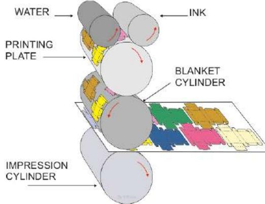
1. The printing plate has the image to be printed on its surface (the image stands out slightly from the printing plate surface).
